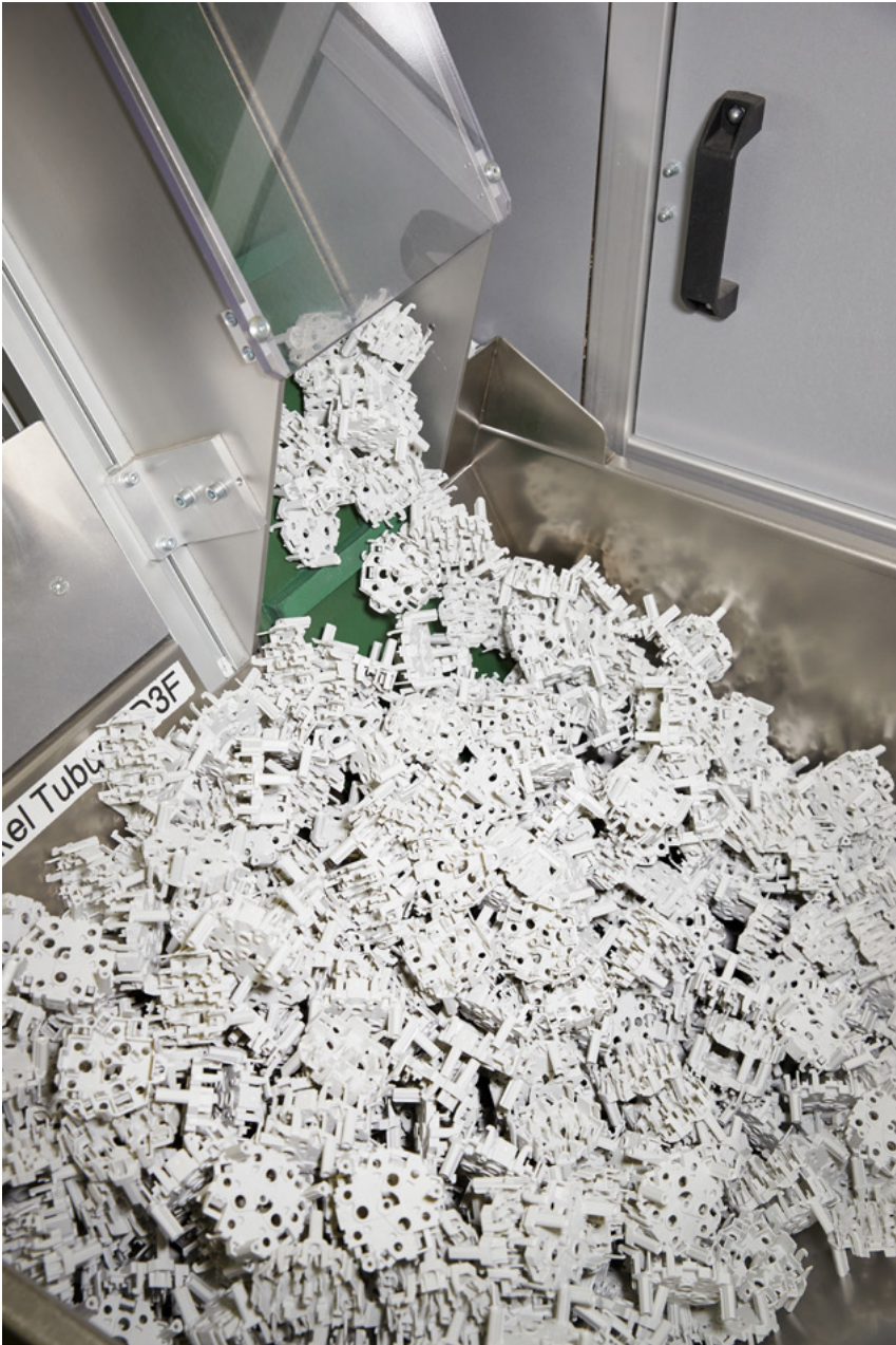
-OUTPUT FROM THE FELLER PLANT IN HORGEN INCLUDES COVER HOUSINGS FOR THREE-FOLD SOCKET OUTLETS AND MOUNTING PLATES
